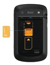
Slide the SIM card into the slot.
