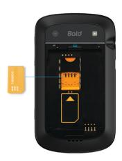
Slide the SIM card into the slot.
