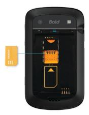
Slide the SIM card into the slot.
