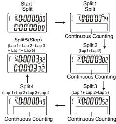
Press button B and then press button A to view different splits records.
