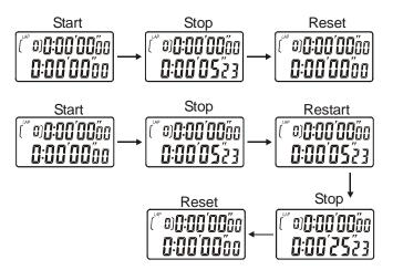
Lap Measurement (Total 30-lap memory measurements and 99-lap measurements). For Example: 5 Laps measurement: Button **D-A-A-A-D**
