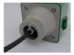
3 - Slide the microphone tubing into the spout and connect the Well Watch to the spout with the plastic ring nut.
