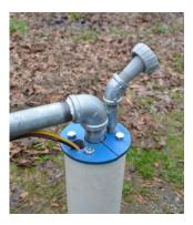
2 - Press the microphone tube into the small hole where the spout attaches. The tube should be long enough to reach through all of the fittings and reach approximately 1" into the well cavity. The tube can be extended up to 6ft. The tubing is 1/4" OD PE and is available at most hardware stores if additional tubing is required.
